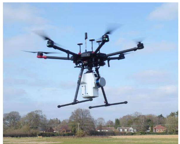
Figure 10: Hyperspectral and lidar capable drone, deployed at Rothamsted since 2021
