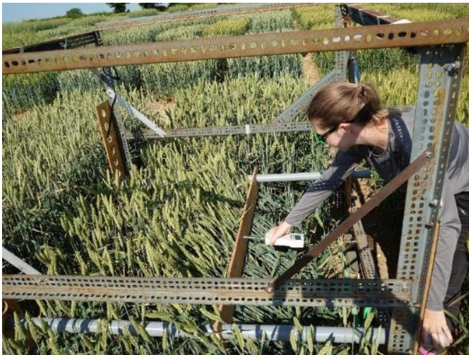
Figure 4: Push-O-Meter v2; device for measuring plot strength.
