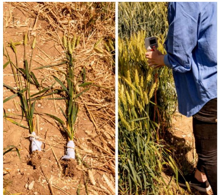
Figure 6: "Pull-O-Meter" v2; device for measuring root anchorage
